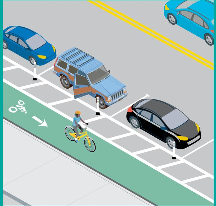
Figure 28. Cycle track protected by paint and soft-hit posts.
