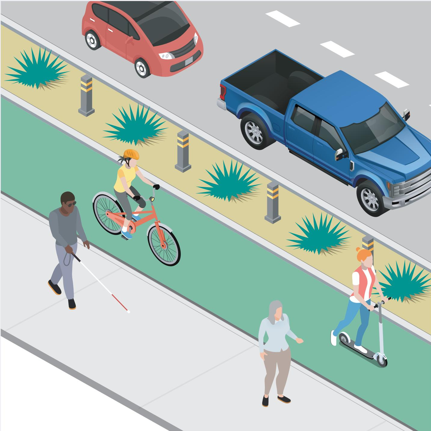
Figure 4. Cycle track protected by a median with plantings.
